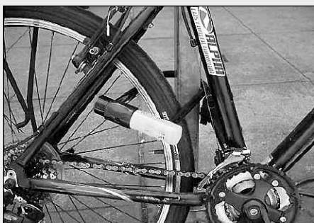
Better, by locking your back wheel inside the rear triangle, you protect your wheel and the frame. It's nearly impossible to cut the rim of a wheel. Just make sure your lock is around the rim and through the triangle. Bonus hint: Front wheels are cheap- back wheels have special gears and cost about twice as much, so if you can to only protect one wheel, make it the back one!
